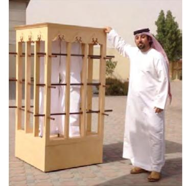
By using the same architectural design, I used the four side entries to keep the air moving from one side to others. Then, I removed the cross wall in the middle and replaced that with a vertical axis rotor. The shape of this rotor was designed specially for this type of wind turbine so with small amount of air, the rotor will start moving to convert this action to generate electricity.
